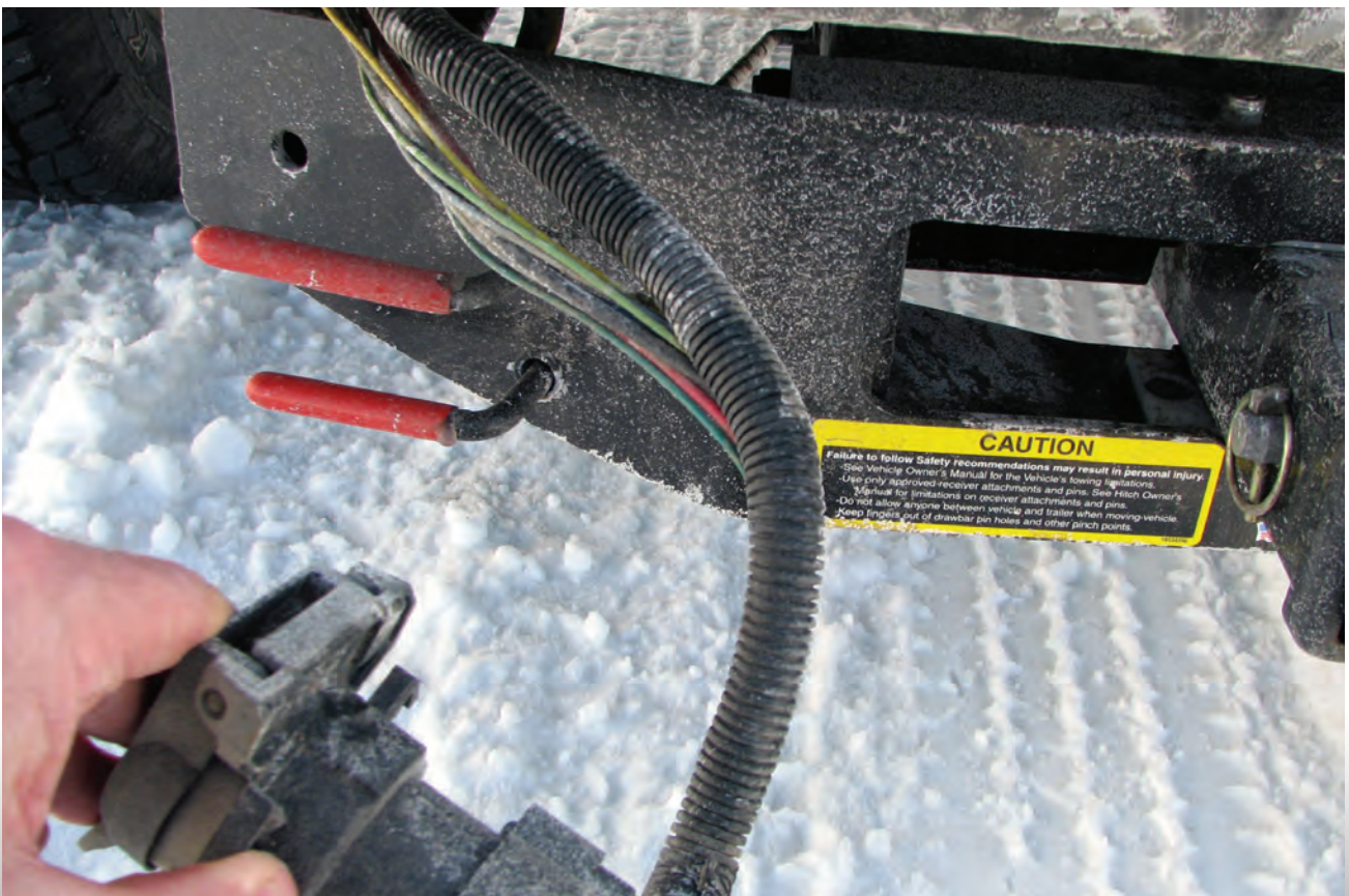
Electric trailer brakes can only work if you properly maintain the wires and plug-ins. Broken covers or split wire housings can lead to brake and light failures.
