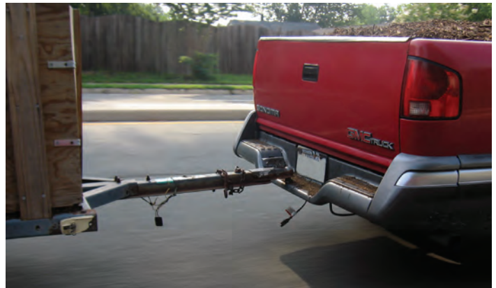
This truck is pulling a trailer without safety chains, plus the lights and brakes are disconnected.
