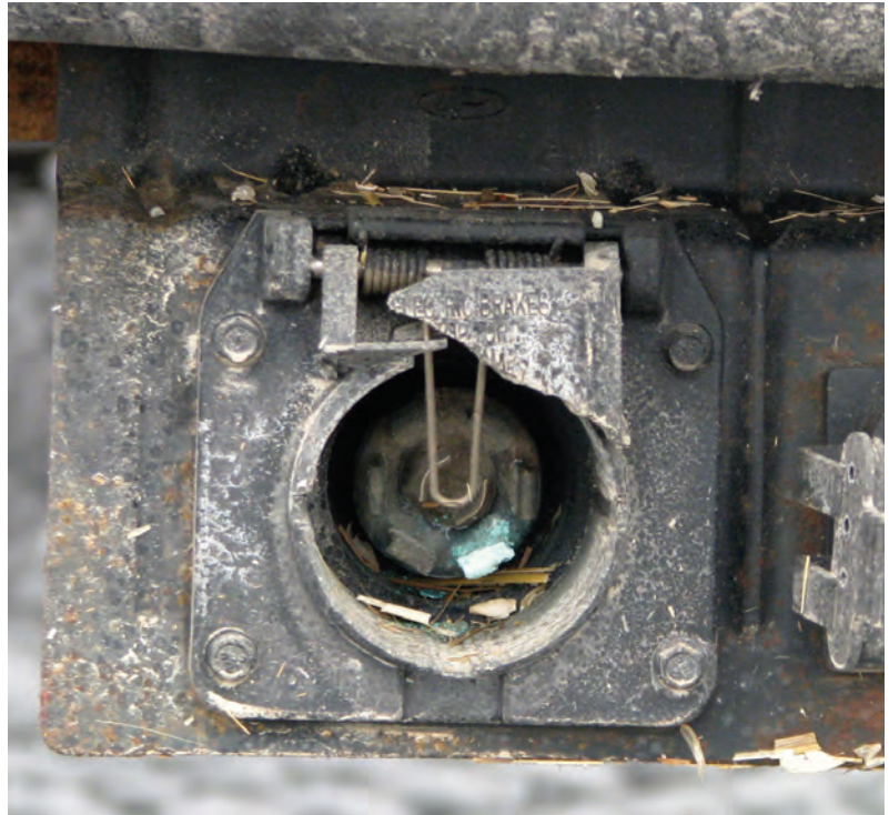
Electric trailer brakes can only work if you properly maintain the wires and plug-ins. Broken covers or split wire housings can lead to brake and light failures.
