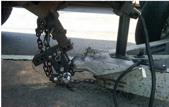
This receiver bent after being sideswiped by another truck.
