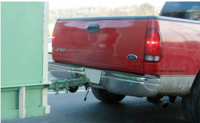
This truck is pulling a trailer without safety chains.
