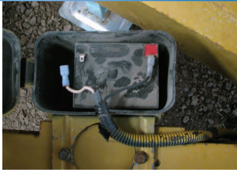
Make sure to occasionally inspect the control box to ensure that the wiring is intact.
