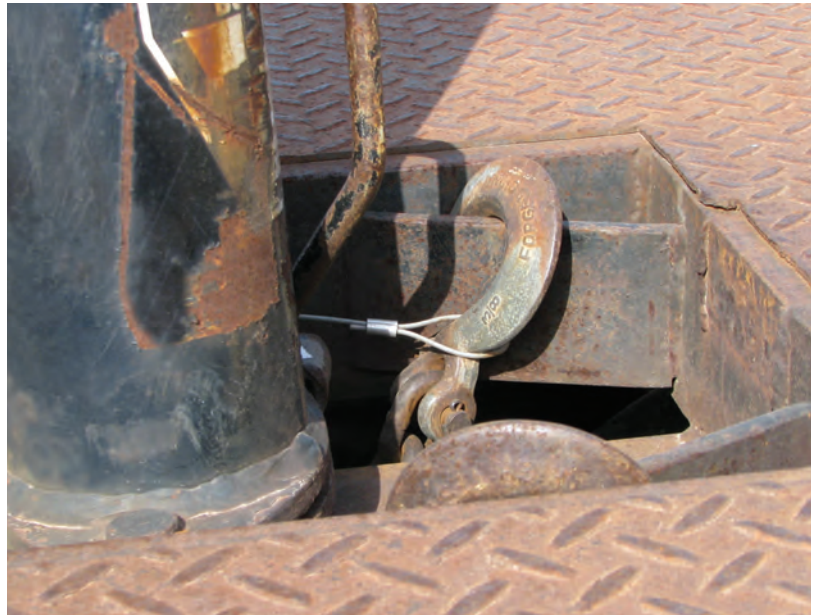
(Above) This emergency cable is improperly attached to the safety chain. (Below right) This truck has an attachment point dedicated to the emergency brake cable. (Below left) This emergency brake cable is in good working condition.
