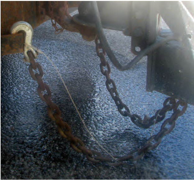
This emergency trailer brake cable is improperly hooked to the chain.
