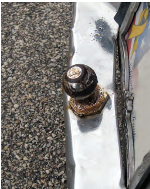
Pulling a trailer that is too heavy can pull the bumper and ball back toward the trailer.
