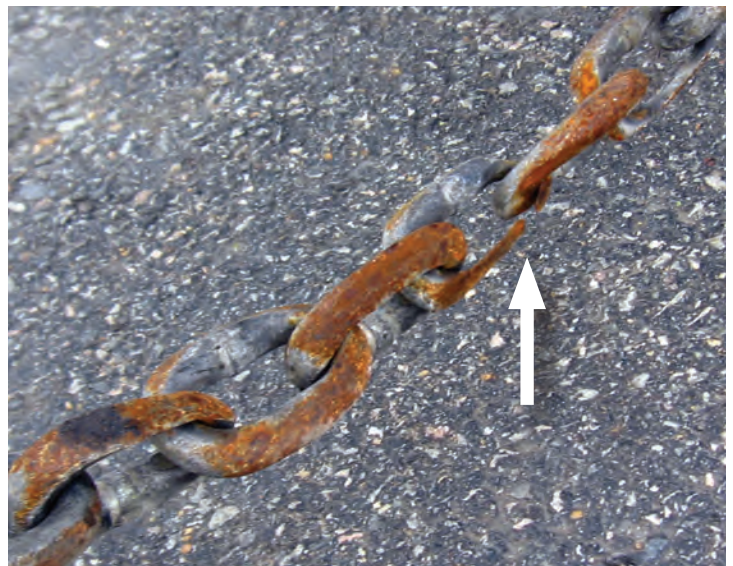
Make sure that safety chains are in good condition. This chain is so corroded that there is a good chance it could break if the trailer came loose.
