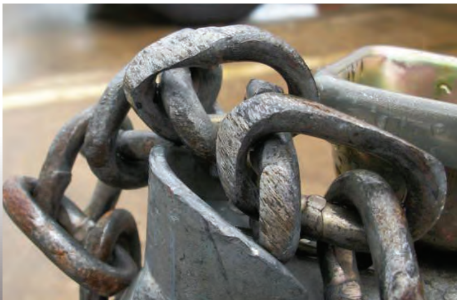
A chain that is too long will drag on the pavement, which weakens the chain.
