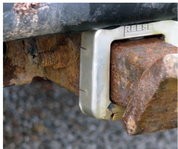
A hitch pin that has rusted in place (bottom), and one designed to be locked (top).
