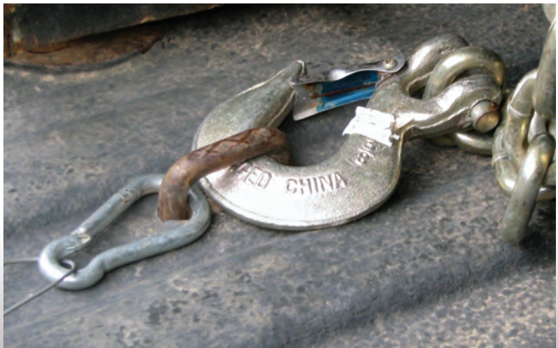
(Above) This emergency cable is improperly attached to the safety chain. (Below right) This truck has an attachment point dedicated to the emergency brake cable. (Below left) This emergency brake cable is in good working condition.
