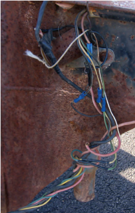
Electric trailer brakes can only work if you properly maintain the wires and plug-ins. Broken covers or split wire housings can lead to brake and light failures.
