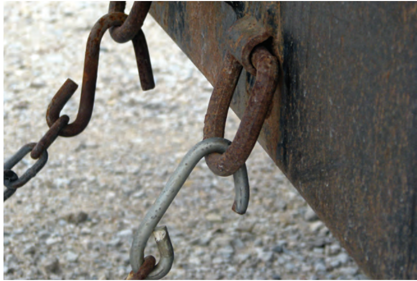
This is a great attachment point, but that benefit is negated by using a hook that has been stretched to the point that it serves no useful function.
