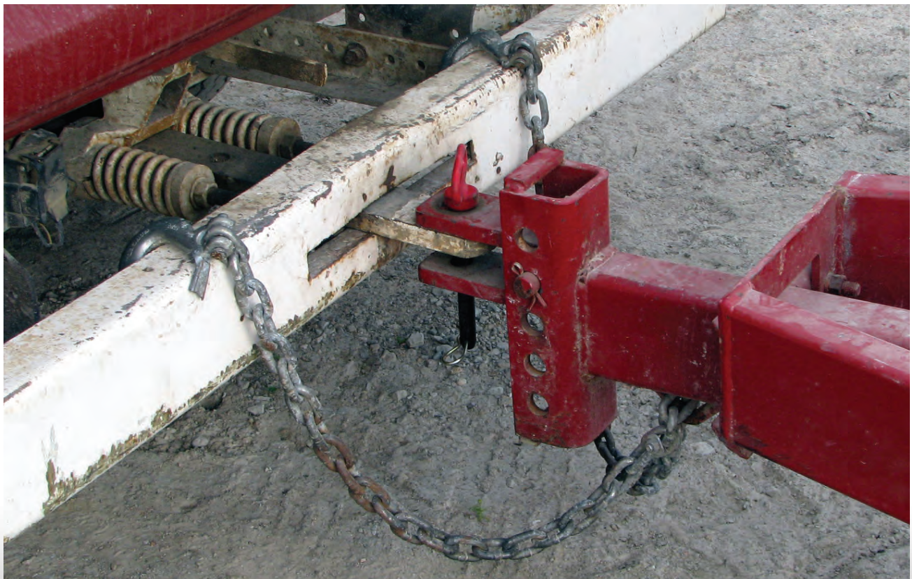
On the left side of this bumper, you can see that the driver broke off the spring-loaded backs of the hooks on the safety chain.
