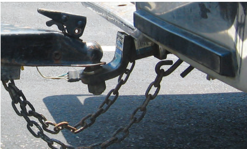
Don't forget the details. This coupler latch does not have a pin to keep it attached to the ball.
