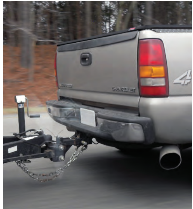
This truck has safety chains that have been properly criss-crossed.
