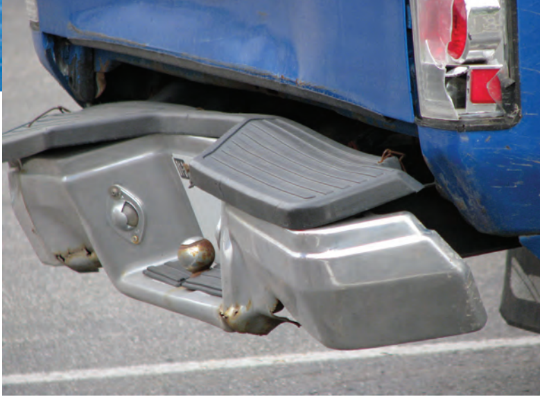
These bumpers have been twisted from towing excess weight.
