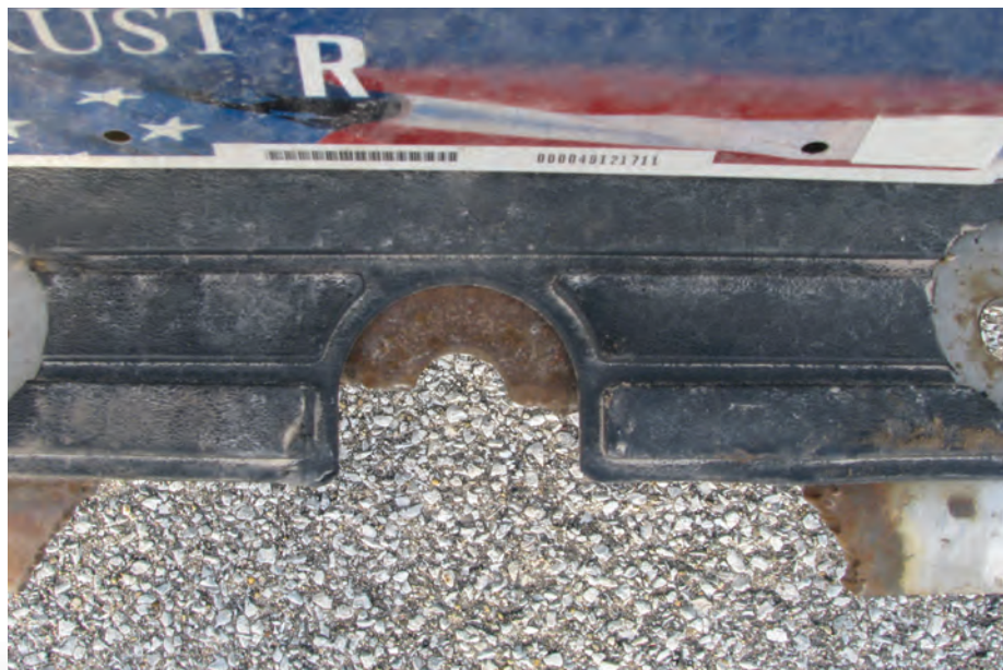
When a trailer is too heavy, it can pull the ball right off the bumper.
