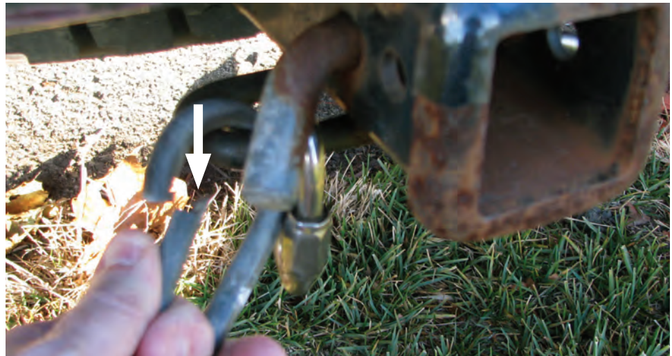
This is a great attachment point, but that benefit is negated by using a hook that has been stretched to the point that it serves no useful function.
