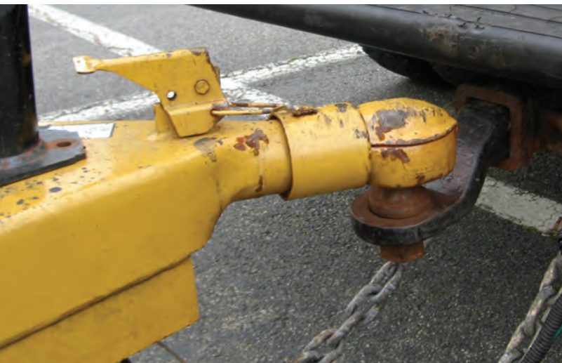
On this trailer the coupler latch pin is not in place.
